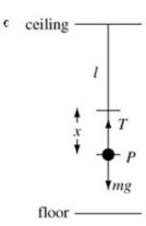
The maximum speed occurs when the acceleration is zero. Let the extension of the string at this point be x.
