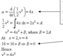
When the acceleration is a function of the displacement, x metres, you write  $a = \frac{d}{dx} \left( \frac{1}{2} v^2 \right)$  and integrate both sides of the equation with respect to x.
