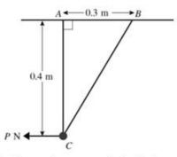
The figure shows a particle C of mass 2 kg suspended by two strings. The strings are fixed to two points A and B on a horizontal ceiling, where  $AB = 0.3 \,\mathrm{m}$ . The string ACis light and inextensible, with length 0.4 m, while the string BC is light and elastic with natural length 0.4 m and modulus of elasticity 32 N. A horizontal force of magnitude P N holds the system in equilibrium with AC vertical.
