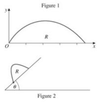
A uniform prism P has cross section R. The prism is placed with its rectangular face on a slope inclined at an angle  $\theta$  to the horizontal. The cross section R lies in a vertical plane as shown in Figure 2. The surfaces are sufficiently rough to prevent P
