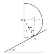
The diagram shows the centre of mass G above the point of contact S.
