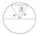
The moment of inertia of the sphere about a diameter  $=\frac{2}{5}ma^2$ This is true for any diameter and in particular for a diameter parallel to the chord. Let *I* be the moment of inertia of the sphere about the chord, which is a distance  $\frac{a}{\sqrt{2}}$  from *O*
