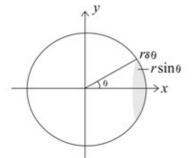
Divide the sphere into hoops one of which is shown. The surface area of the hoop =  $2\pi r \sin \theta \times r \delta \theta$
