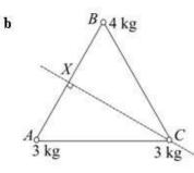
Let X be mid-point of AB Total M.I. about  $CX = 3x \left(\frac{a}{2}\right)^2 + 4x \left(\frac{a}{2}\right)^2 + 3x 0$   $= \frac{3a^2}{4} + \frac{4a^2}{4}$ M.I. $_{\alpha} = \frac{7a^2}{4}$
