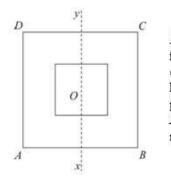
A uniform lamina of mass m is formed from a square lamina ABCD of side 2a by cutting out a square of side a. Both squares have the same centre O and their sides are parallel as shown in the figure. The points X and Y are the mid-points of AB and CDrespectively.
