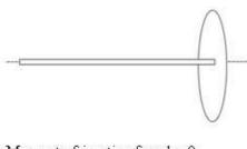
Moment of inertia of rod = 0Moment of inertia of  $disc = \frac{1}{2}mr^2$  $\therefore$  Total M.  $I = \frac{1}{2}mr^2$
