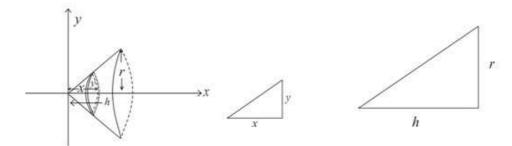
Divide the cone into thin discs – one of which is shown. Its mass is  $\delta m$ , its thickness is  $\delta x$ , its radius is y and it is at a distance x from the y-axis.
