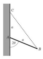
A uniform  $\operatorname{rod} AB$ , of mass m and length a, can rotate in a vertical plane about a smooth hinge fixed at A on a vertical wall. A point C on the wall is at a height a vertically above A. One end of an elastic string, of natural length a and modulus of elasticity 2mg, is attached to C and the other end is attached to the end B of the rod, as shown in the diagram.
