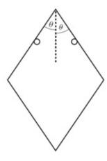
Four equal uniform rods each of length 2a and mass m are smoothly jointed to form a rhombus. This is used by a gardener to measure areas of lawn for treatment. When not in use it is stored resting on two smooth pegs, which are at the same level and a
