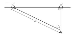
A uniform rod PQ has mass m and length 2l. A smooth light ring is fixed to the end P of the rod. This ring is threaded on to a fixed horizontal smooth straight wire. A second small smooth light ring R is threaded on to the wire and is attached by a light elastic string, of natural length l and modulus of elasticity kmg, to the end Q of the rod, where k is a constant.
