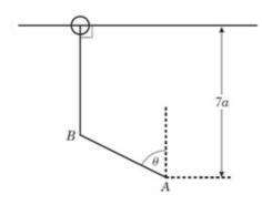
A uniform rod AB, of length  $2\alpha$  and mass 8m, is free to rotate in a vertical plane about a fixed smooth horizontal axis through A. One end of a light elastic string, of natural
