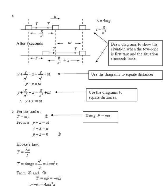
Auxiliary equation:  $m^2 + 4n^2 = 0$   $m = \pm 2in$ General solution:  $x = A\cos 2nt + B\sin 2nt$   $t = 0 \quad x = 0 \Rightarrow A = 0$ Tow-rope slack when x = 0  $0 = B\sin 2nt$   $\sin 2nt = 0$   $nt = \pi$ Value of B not needed here.
