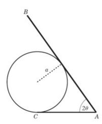
The diagram shows a uniform rod AB, of mass m and length 4a, resting on a smooth fixed sphere of radius a. A light elastic string, of natural length a and modulus of elasticity  $\frac{3}{4}mg$ , has one end attached to the lowest point C of the sphere and the other end attached to A. The points A, B and C lie in a vertical plane with  $\angle BAC = 2\theta$ , where  $\theta < \frac{\pi}{4}$ .
