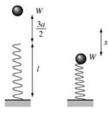
Using conservation of energy, P.E. loss of W = E.E. gain of spring
