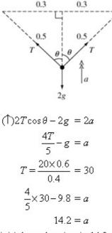
initial acceleration is  $14.2 \text{ m s}^{-2}$  upwards
