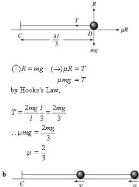
work done against friction = over all loss in energy = E.E. loss - K.E. gain
