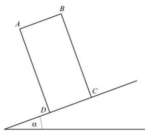
A thin uniform rectangular metal plate ABCD of mass M rests on a rough plane inclined at an angle  $\alpha$  to the horizontal. The plate lies in a vertical plane containing a line of greatest slope of the inclined plane, with the edge CD in contact with the plane and C further up the plane than D, as shown in the figure. The lengths of AB and BC are 10 cm and 30 cm respectively. The plane is sufficiently rough to prevent the plate from slipping.
