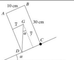
When the system is on the point of toppling about D, the centre of mass of the plate and stud combined, G, is vertically above O.
