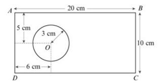
The figure shows a metal plate that is made by removing a circle of centre O and radius 3 cm from a uniform rectangular lamina ABCD, where AB = 20 cm and BC = 10 cm. The point O is 5 cm from both AB and CD and is 6 cm from AD.
