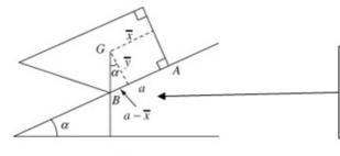
When the lamina is on the point of overturning about B, the centre of mass G of the lamina is vertically above B.
