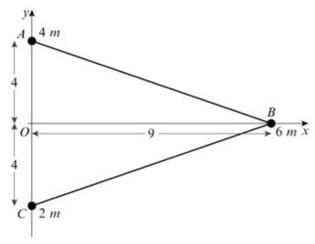
The figure shows a triangular lamina ABC. The coordinates of A, B and C are (0, 4), (9, 0) and (0, -4) respectively. Particles of mass 4m, 6m and 2m are attached at A, B and C respectively.
