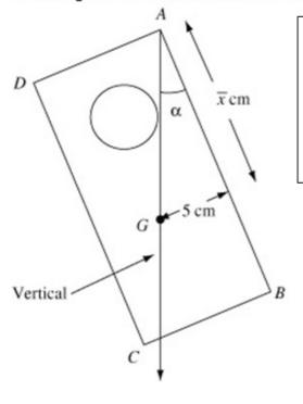
When the plate is suspended freely from A, its centre of mass G is vertically below the point of suspension A. The distance of G from AD was found in  $\mathbf{a}$  and the distance of G from AB is 5 cm by symmetry. You calculate  $\alpha$  using trigonometry.
