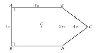
The figure shows a uniform lamina ABCDE such that ABDE is a rectangle, BC = CD, AB = 8a and AE = 6a. The point X is the mid-point of BD and XC = 4a. The centre of mass of the lamina is at G.
