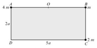
A loaded plate L is modelled as a uniform rectangular lamina ABCD and three particles. The sides CD and AD of the lamina have length 5a and 2a respectively and the mass of the lamina is 3m. The three particles have mass 4m, m and 2m and are attached at the points A, B and C respectively, as shown in the figure.
