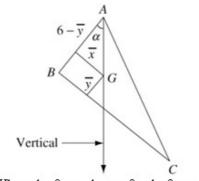
When the frame hangs freely from A, its centre of mass G is vertically below A.
