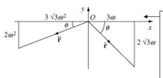
A diagram is essential here. Once the diagram has been drawn, the problem reduces to basic trigonometry. You find the angles using the inverse tangent button on your calculator. The final angle could be given in degrees or radians (1.92°).
