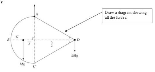
M(A),  $Mg\overline{x} = kMg \times \frac{3}{2}$  $\Rightarrow k = \frac{2}{3} \times \frac{23}{6(2\pi + 3)}$   $= \frac{23}{9(2\pi + 3)} = 0.275 (3 \text{ s.f.})$ Taking moments about A means we don't need to know the force A.
