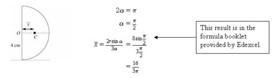
Centre of mass is on the axis of symmetry at a distance
