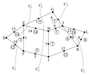
The diagram shows a network of roads represented by arcs. The capacity of the road represented by that arc is shown on each arc. The numbers in circles represent a possible flow of 26 from B to L.
