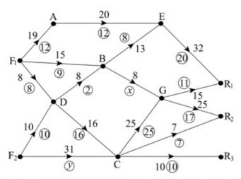
The diagram shows a capacitated, directed network of pipes flowing from two oil fields  $F_1$  and  $F_2$  to three refineries  $R_1$ ,  $R_2$  and  $R_3$ . The number on each arc represents the capacity of the pipe and the numbers in the circles represent a possible flow of 65.
