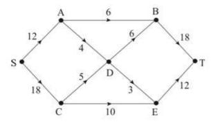
The diagram shows a capacitated network. The numbers on each arc indicate the capacity of that arc in appropriate units.
