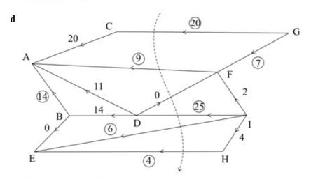
e Max flow - min cut Finds a cut GC, AF, DF, DI, EI, EH value 64 Note: must not use supersource or supersink arcs.
