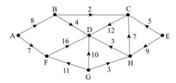
The network above models a drainage system. The number on each arc indicates the capacity of that arc, in litres per second.
