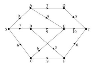
The network shows possible routes that an aircraft can take from S to T. The numbers on the directed arcs give the amount of fuel used on that part of the route, in appropriate units. The airline wishes to choose the route for which the maximum amount of fuel used on any part of the route is as small as possible. This is the minimax route.
