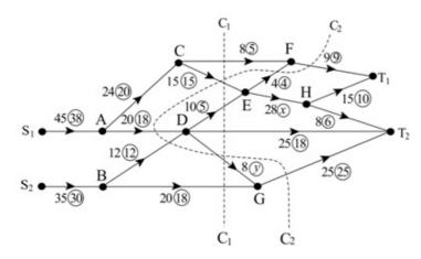
The diagram shows a capacitated, directed network. The unbracketed number on each arc indicates the capacity of that arc, and the numbers in circles show a feasible flow of value 68 through the network.
