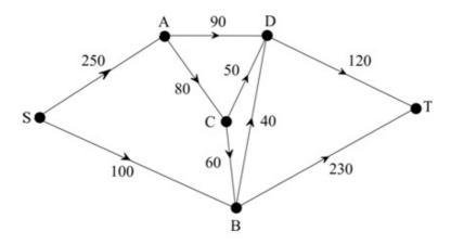
Natural gas is produced at S and is transported to a refinery at T by a network of underwater pipelines. The capacity of each pipeline, in appropriate units, is given in the diagram which shows the network of pipelines
